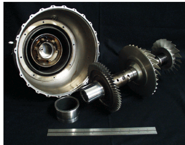
Fig. 1. WJ24-8 rotor, aft housing and MiTi ® air foil bearing after engine demonstration test.
