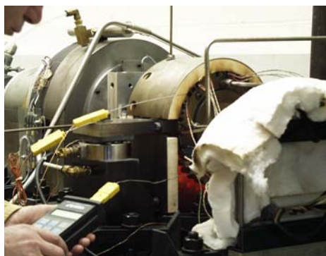
Figure 1 Test Rig with a 150 mm Magnetic Bearing and a 150 mm Foil Bearing
