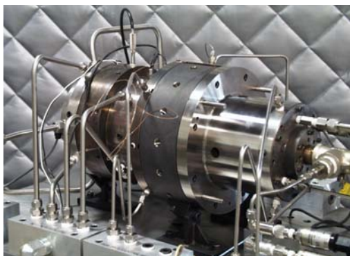
Figure 1. High temperature foil thrust rig.
