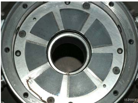
Figure 3. Advanced high load thrust foil bearing.
