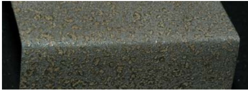
Figure 1. MiTi® Korolon™ 1350A coating adhesion bend test without delamination.
