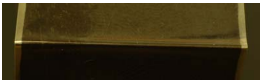
Figure 2. MiTi® Korolon™ 1350B coating adhesion bend test without delamination.
