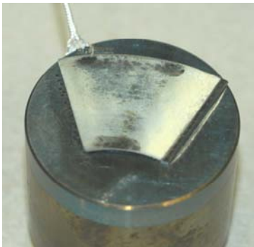
Figure 10. Pad with a composite coating after a high temperature test against a disk coated with hard chrome.
