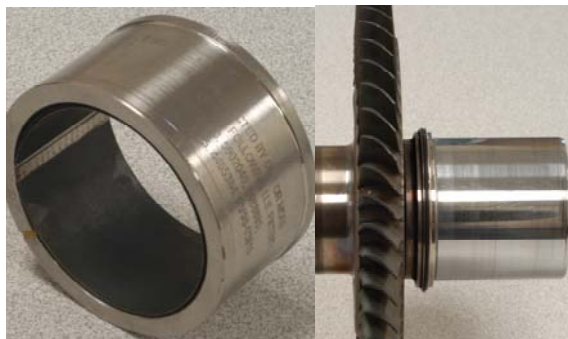
Figure 11. Foil bearing and journal after engine testing.
